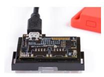
Figure 4. CC1350STK with attached DevPack board
